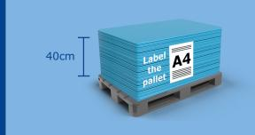
Each pallet of PLPs must be stacked evenly to a height of approximately 40cm and labelled properly for traceability.
