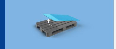
Make sure to remove the last plastic layer pad (PLP) from the pallet.
