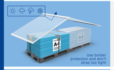
**Note:** Too much tension can cause damage to the PLPs. To avoid damages by strapping too tight, secure the pallet with a top frame or border protection and band with plastic straps. Pallets may otherwise be secured and packed with shrinking foil.
