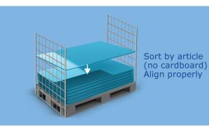
Ensure that PLPs are aligned with the pallet and stacked correctly to prevent collapse and risk of damage by irregular stacking.
